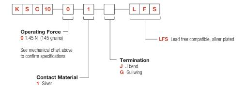
Note: KSC10 offered with yellow actuator as standard, hardness 55 Shore
